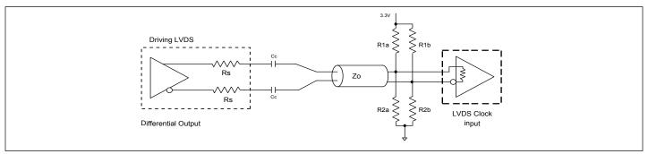
Figure 2. Differential Output Driving LVDS
