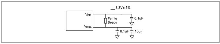
Figure 3. Power Supply Filter
