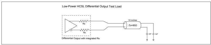
Figure 1. Low Power HCSL Test Circuit
