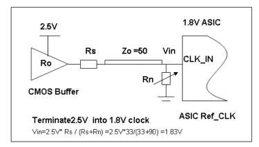
Rs = 33 ohm with Rn = 100 ohm, to transition 3.3V CMOS to 2.5V Rs = 43 ohm with Rn =70 ohm to transition 3.3V CMOS to 1.8V
