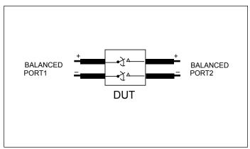
Fig 1. Differential Insertion Loss Setup
