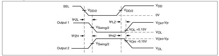
**Voltage Waveforms Enable and Disable Times**
