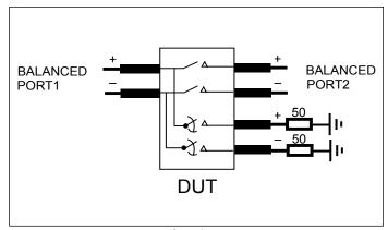
Fig 2. Off-isolation Setup
