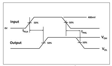
Fig 4. Propagation Delay
