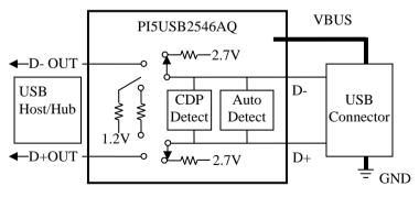
Figure 2c, Divider-2.4A Charging Scheme
