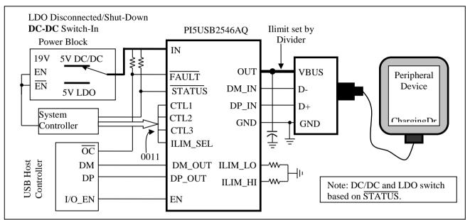
Figure 7, Case 1: System in S4/S5, Device Charging
