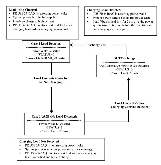
Figure 6, PI5USB2546AQ Power Wake flow chart
