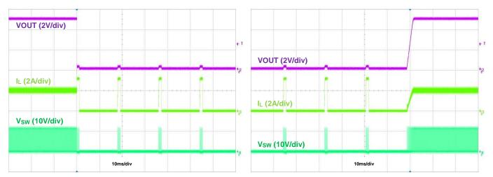
Figure 23. Output Short Protection, IOUT = 2A
