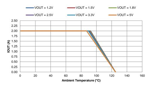
Figure 26. Output Current Derating Curve vs. Ambient Temperature, VIN = 12V, fsw = 500kHz
