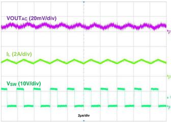
Figure 15. Output Voltage Ripple, VOUT = 5V, IOUT = 2A
