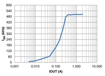
Figure 13. fsw vs. Load
