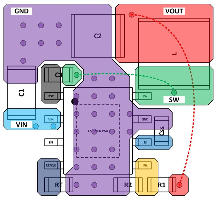
Figure 28. Recommended PCB Layout
