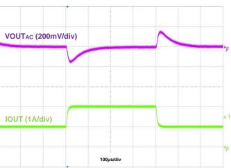
Figure 19. Load Transient, IOUT = 1A to 2A to 1A
