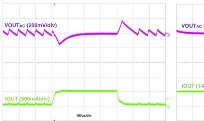
Figure 18. Load Transient, IOUT = 50mA to 500mA to 50mA
