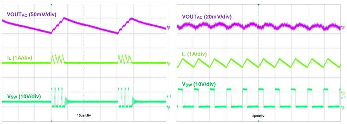
Figure 16. Output Voltage Ripple, VOUT = 3.3V, IOUT = 50mA
