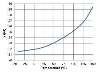
Figure 10. IQ vs. Temperature
