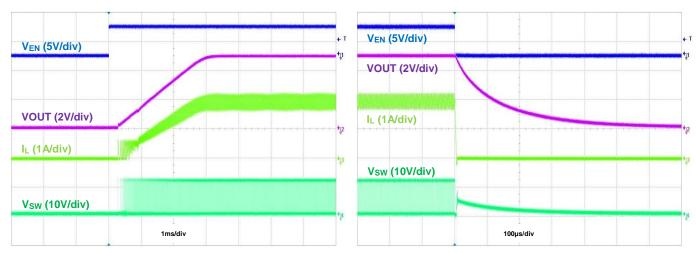
Figure 21. Startup Using EN, IOUT = 2A
