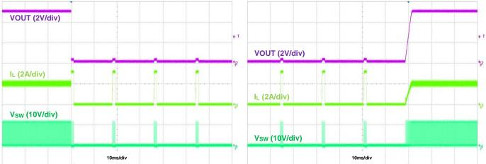
Figure 23. Output Short Protection, IOUT = 2A
