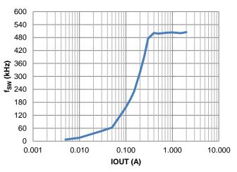
Figure 13. fsw vs. Load
