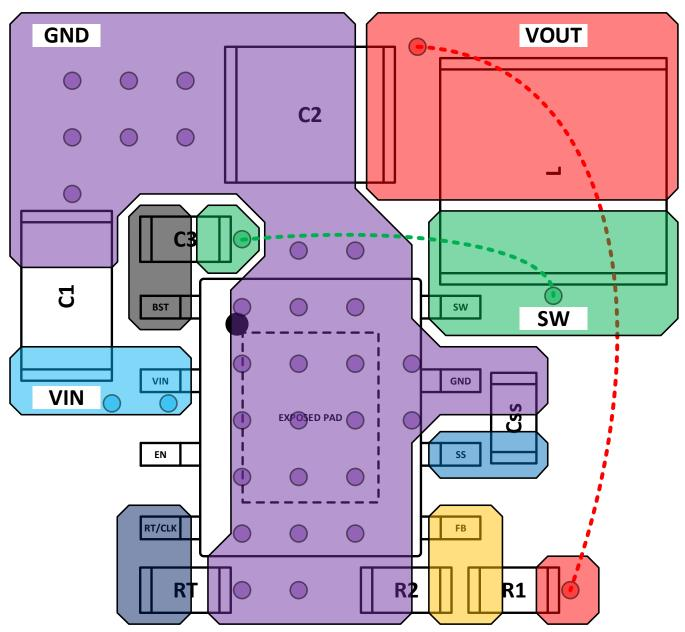
Figure 28. Recommended PCB Layout
