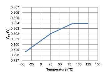
Figure 8. Feedback Voltage vs. Temperature
