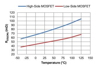
Figure 9. Power MOSFET RDS(ON) vs. Temperature
