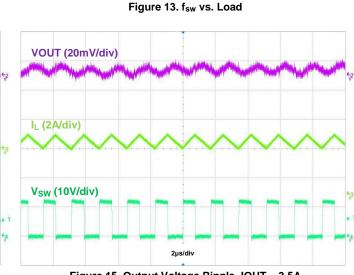
Figure 15. Output Voltage Ripple, IOUT = 3.5A
