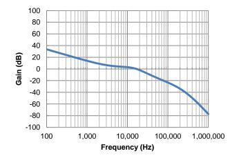
Figure 29. Closed-Loop Bandwidth
