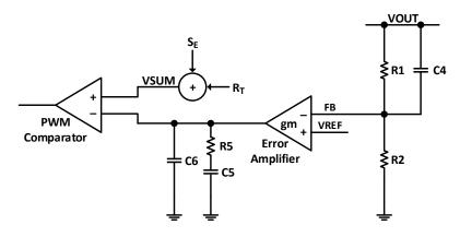
Figure 26. Type II Compensator
