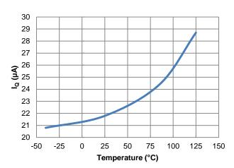
Figure 10. I<sub>Q</sub> vs. Temperature
