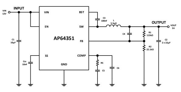
Figure 27. Example Circuit for Loop Compensation Calculations
