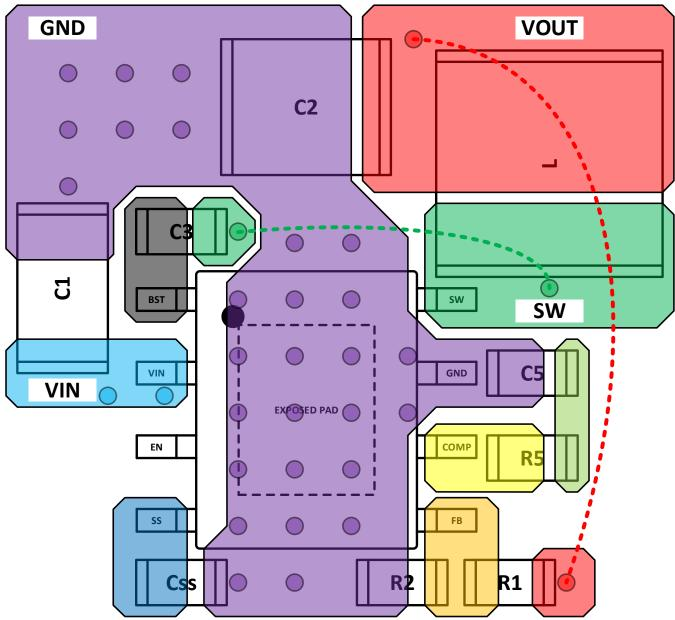
Figure 31. Recommended PCB Layout
