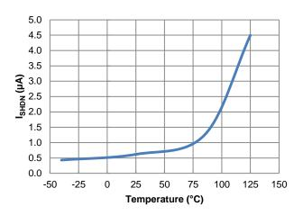
Figure 11. I<sub>SHDN</sub> vs. Temperature
