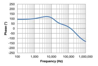
Figure 30. Closed-Loop Phase Margin
