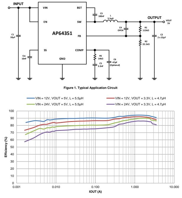
Figure 2. Efficiency vs. Output Current
