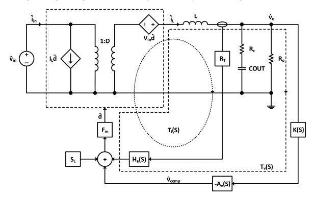
Figure 25. Small Signal Model of Buck Regulator
