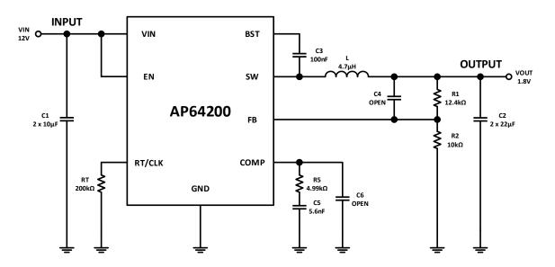
Figure 31. Example Circuit with Calculated Component Values for Loop Compensation
