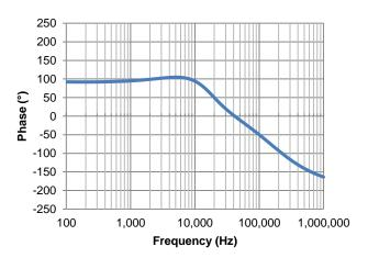
Figure 33. Closed-Loop Phase Margin
