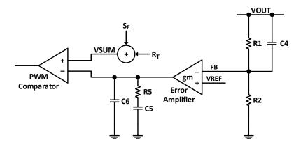
Figure 29. Type II Compensator
