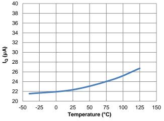
Figure 10. IQ vs. Temperature
