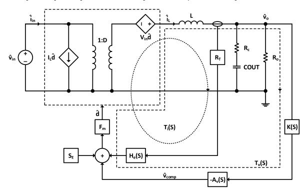
Figure 28. Small Signal Model of Buck Regulator
