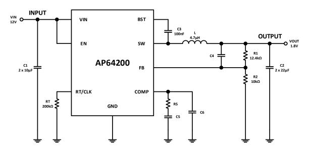
Figure 30. Example Circuit for Loop Compensation Calculations
