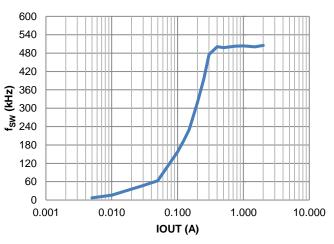
Figure 13. fsw vs. Load
