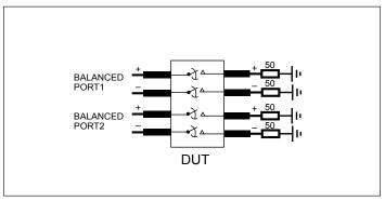
Differential Near End Xtalk Test Circuit
