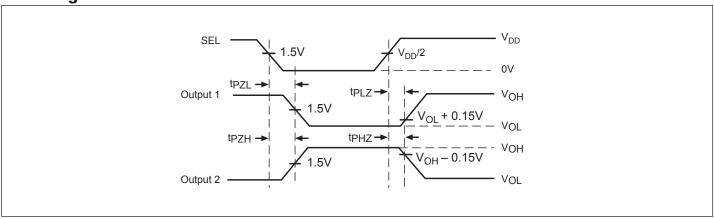
**Voltage Waveforms Enable and Disable Times**
