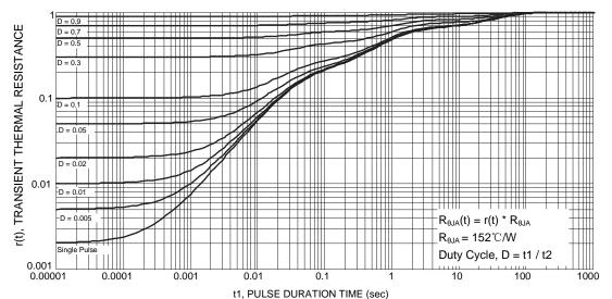
Figure 13 Transient Thermal Resistance
