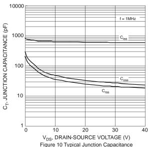
Figure 10 Typical Junction Capacitance
