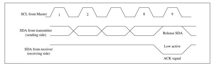
After transmitting the ACK signal, if the Master remains the receiver for transfer of the next byte, the SDA is released at the falling edge of the clock corresponding to the 9th bit of data on the SCL line. Data transfer resumes when the Master becomes the transmitter.
