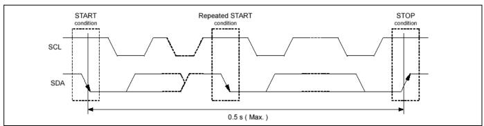
Fig.2 Starting and stopping on I<sup>2</sup>C bus
