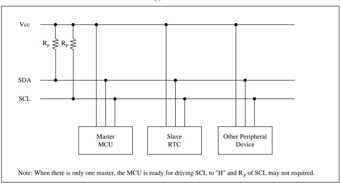
Fig.1 System configuration
