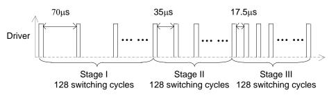
Figure 4. Driver Time Sequence in Startup Process
