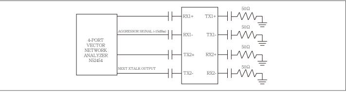
Figure 4. Channel-Isolation Test Configuration
