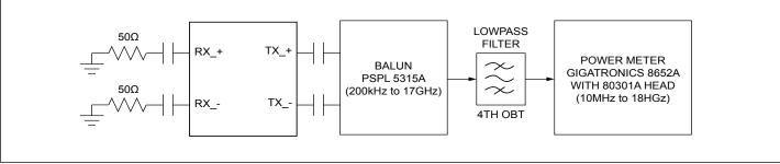
**Figure 5. Noise Test Configuration**
