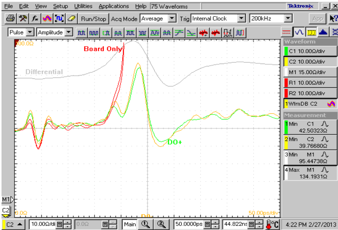
Figure 8. TDR Channel D0, VDD=3.0V, 25C
