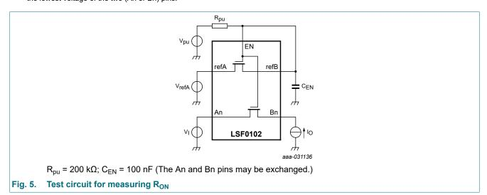
2-bit bidirectional multi-voltage level translator; open-drain; push-pull
