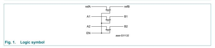
2-bit bidirectional multi-voltage level translator; open-drain; push-pull
