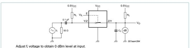
Fig. 21. Test circuit for measuring isolation (OFF-state)
