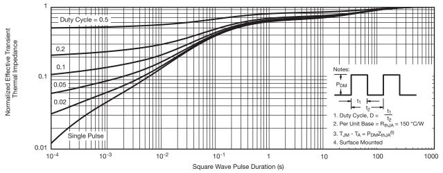
Normalized Thermal Transient Impedance, Junction-to-Ambient
