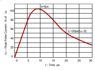
Fig 1.Pulse Waveform
