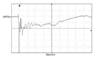
ESD clamping (+8kV contact discharge per IEC61000-4-2)
