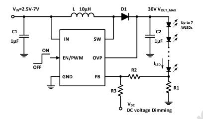
Figure 4. Dimming Control by a DC Voltage
