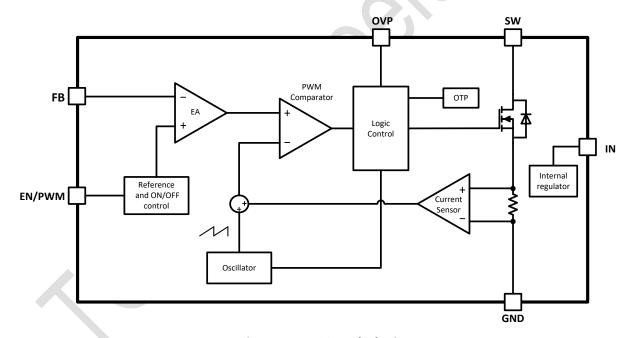
Figure 2. STI9287B Block Diagram
