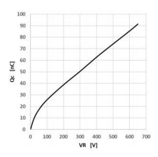
Figure 6 Capacitance Charge vs. Reverse Voltage
