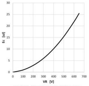
Figure 7 Capacitance Stored Energy
