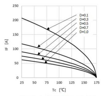
Figure 3 Peak Forward Current Derating
