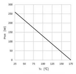
Figure 4 Power Dissipation
