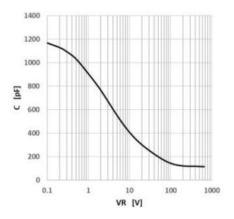
Figure 5 Capacitance vs. Reverse Voltage
