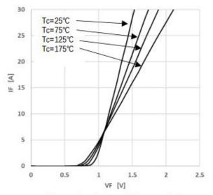
Figure 1 Forward Characteristics
