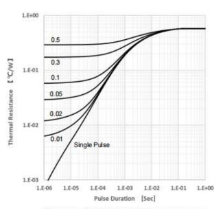
Figure 8 Transient Thermal Impedance
