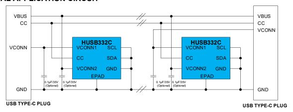
Figure 1. HUSB332C\_B44DA Typical Application Circuit
