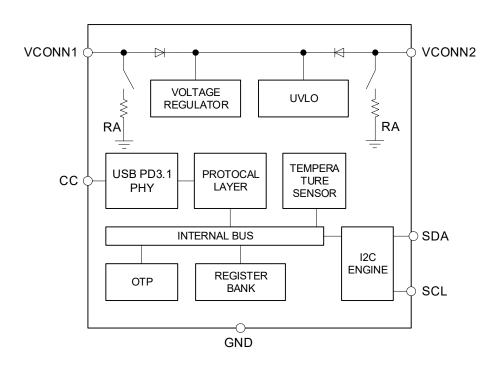
Figure 3. HUSB332C Functional Block Diagram
