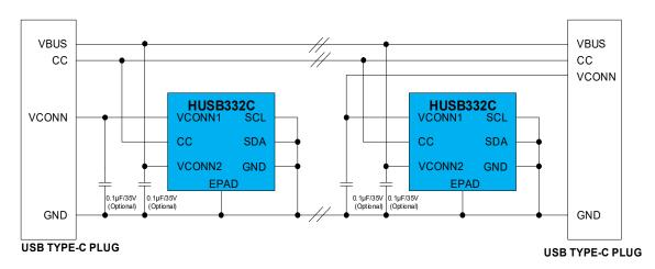
Figure 8. Two eMarkers Solution without VCONN Connected Through the Cable
