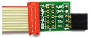
Figure 3. USB-I2C-ADPTZ Adapter Board
