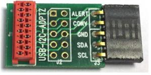
Figure 4. USB-I2C5W-ADPTZ Adapter Board
