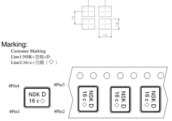
The inner vision of Pin#1, Pin#4 side is XTAL blank mounting pad.
