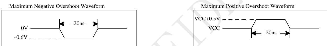
Figure 5-1 Maximum Overshoot Waveform
