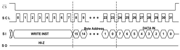
Figure 10: WRITE Timing
