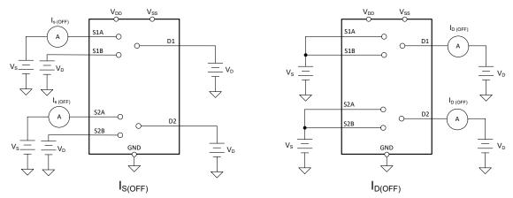
Figure 7-2. Off-Leakage Measurement Setup
