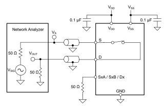
Figure 7-12. Bandwidth Measurement Setup
