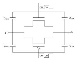
Figure 8-1. Transmission Gate Topology
