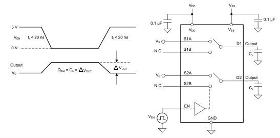
Figure 7-9. Charge-Injection Measurement Setup
