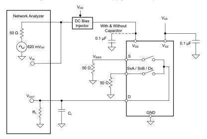
Figure 7-14. ACPSRR Measurement Setup
