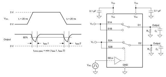
Figure 7-6. Break-Before-Make Delay Measurement Setup
