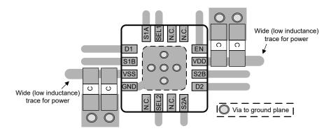
Figure 11-2. TMUX7236 Layout Example
