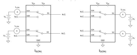
Figure 7-3. On-Leakage Measurement Setup
