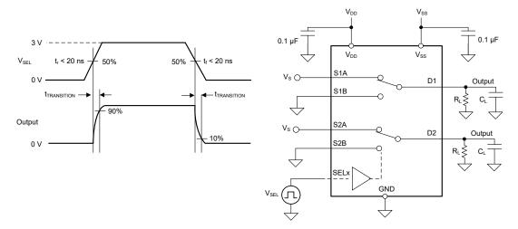
Figure 7-4. Transition-Time Measurement Setup
