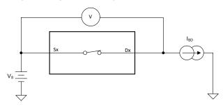
Figure 7-1. On-Resistance Measurement Setup
