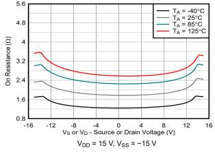
Figure 9-2. On-Resistance vs Temperature
