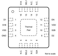
Figure 5-1. RUM Package, 16-Pin WQFN (Top View)
