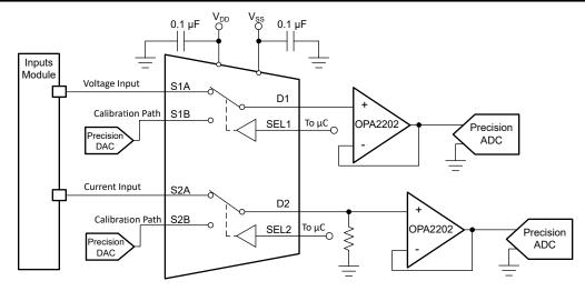
Figure 9-1. Data Acquisition Systems (DAQ) Calibration
