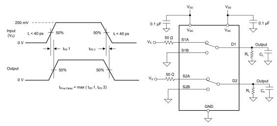
Figure 7-8. Propagation Delay Measurement Setup
