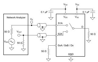
Figure 7-11. Crosstalk Measurement Setup
