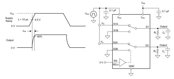
Figure 7-7. t<sub>ON (VDD)</sub> Time Measurement Setup
