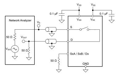
Figure 7-10. Off Isolation Measurement Setup
