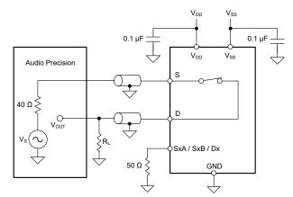
Figure 7-13. THD Measurement Setup
