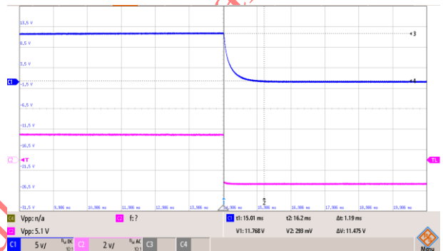
CH1: V OUT CH2:EN EN Shutdown, V IN =48V, I OUT =1A
