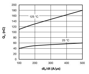
Fig. 8 - Typical Stored Charge vs. dl<sub>E</sub>/dt
