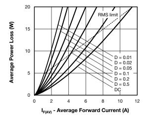
Fig. 6 - Forward Power Loss Characteristics
