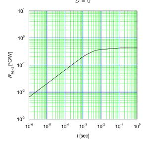
Figure 21. Transient Thermal Impedance of FWD
