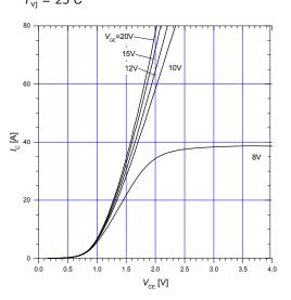
Figure 7. Typical output characteristics  $T_{vj} = 175^{\circ}\text{C}$
