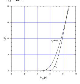
Figure 9. Gate threshold voltage  $I_{\rm C}$  = 40 mA,  $V_{\rm CE}$  = 20 V
