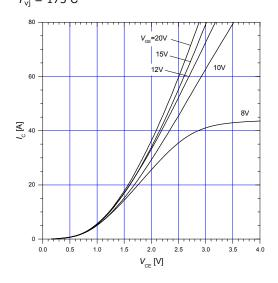
Figure 8. Typical transfer characteristics  $V_{\rm CE}$  = 20 V
