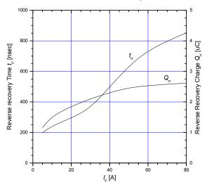
Figure 18. Typical reverse recovery loss vs.  $I_{\rm F}$   $V_{\rm CC}$  = 600 V,  $V_{\rm GE}$  = 15 V,  $R_{\rm G}$  = 10  $\Omega$ ,  $T_{\rm vj}$  = 175°C
