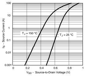
Forward Diode Voltage vs. Temperature
