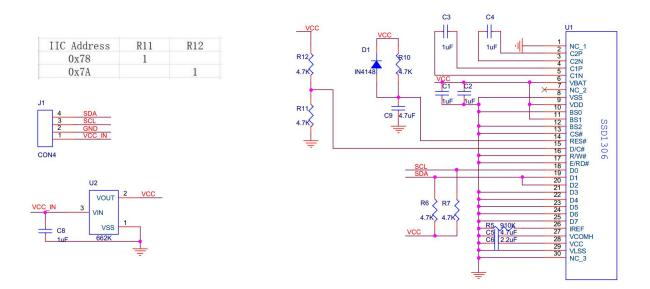
The I2C communication interface consists of slave address bit DC, I2C-bus data signal SDA (SDAOUT/D2 for output and SDAIN/D1 for input) and I2C-bus clock signal SCL (D0). Both the data and clock signals must be connected to pull-up resistors.
