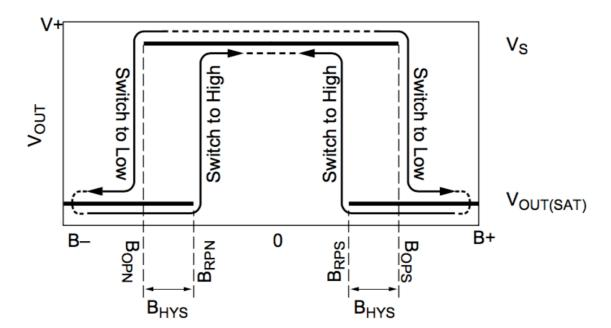
If the device is powered on with a magnetic field strength between B<sub>RP</sub> and B<sub>OP</sub>, then the device output is determinate High. For all packages, if the field strength is greater than B<sub>OP</sub>, then the output is pulled low. If the field strength is less than B<sub>RP</sub>, the output is released.
