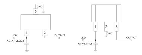
Note: C<sub>IN</sub> is for power stabilization and to strengthen the noise immunity, the recommended capacitance is 0.1~1uF.
