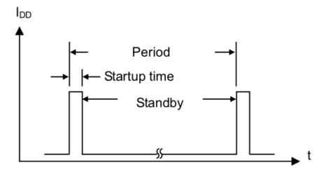
The unipolar detection Hall IC adopts an intermittent operation method to save energy. At startup, the Hall elements, amp, comparator and other detection circuit power ON and magnetic detection begins. During standby, the detection circuits power OFF, thereby reducing current consumption. The detection results are held while standby is active, and then output.
