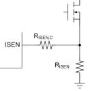
Fig. feed-forward resistor
