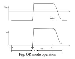
The voltage across drain and source of the MOSFET is reflected by the auxiliary winding of the transformer. VSEN pin detects the voltage across the auxiliary winding by a resistor divider. When the voltage across drain and source of the MOSFET is at voltage valley, the MOSFET would be turned on.
