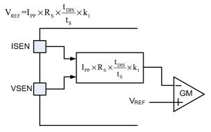
Fig. Output current detection diagram
