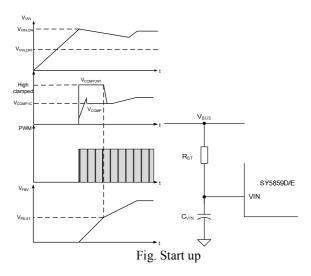
This operation is aimed to build up enough output voltage for auxiliary winding bias supply as quickly as possible. It is enabled only one time just when  $V_{VIN}$  is over  $V_{VIN,ON}$ .
