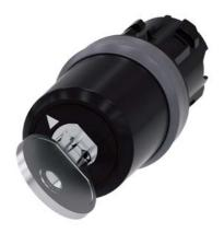
Key-operated switch BKS, 22 mm, round, plastic with metal front ring, lock number S1, with 2 keys, 2 switch positions O-I, latching, actuating angle  $90^{\circ}$ , 10:30h/13:30h, Key removal O+I
