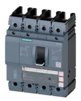
circuit breaker 3VA5 UL frame 250 breaking capacity class M 35kA @ 480 V 4-pole, line protection TM230, FTAM, In=150A overload protection Ir=150A fixed short-circuit protection Ii=5...10 x In N conductor unprotected without connection
