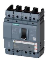
circuit breaker 3VA5 UL frame 250 breaking capacity class H 65kA @ 480V 4-pole, line protection TM230, FTAM, In=250A overload protection Ir=250A fixed short-circuit protection Ii=5...10 x In N conductor unprotected without connection
