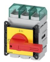
SENTRON, Molded case switch 3LD5 UL, Emergency switching-off, 3-pole, certified according to UL489 UL60947-4-1 and IEC60947-3, UL: 125A, SCCR 65kA at 480VAC, Operating power at 480VAC 3-phase: 75hp, IEC: 125A, Operating power at AC-23A at 400V: 55kW, front-mounted, rotary operating mechanism, red/yellow, 4-hole mounting of the handle, incl. terminal covers for the infeed side
