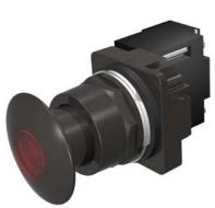
30mm BlackMax, Epoxy Coated Corrosion Resistant Complete Metal Unit Illuminated Push-Pull Operator Transformer type, 120V AC LED Lamp Mushroom Head Cap Small 1 3/4" (44.5 mm) Metal, Black with Red Lens 2 Position Maintained, Pull-to-Release UL Listed, CSA Certified NEMA 1,3,3R,4,4X,12,13 & Automotive Standards
