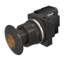
30mm BlackMax, Epoxy Coated Corrosion Resistant Complete Metal Unit Illuminated Push-Pull Operator Transformer type, 240V AC LED Lamp Mushroom Head Cap Small 1 3/4" (44.5 mm) Metal, Black with Amber Lens 2 Position Maintained, Pull-to-Release UL Listed, CSA Certified NEMA 1,3,3R,4,4X,12,13 & Automotive Standards
