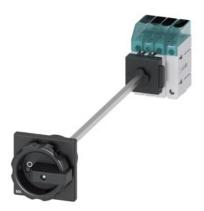
Load disconnector 3LD3, lu 63 A Main switch 3-pole + N Rated operating capacity at AC-23 A at 400V 22.0 kW floor mounting Basic switch with door coupling Central hole mounting 22.5mm Rotating drive black 66 x 66 mm
