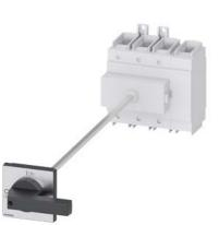
SENTRON, Switch disconnector 3LD, main switch, 4-pole, lu=250 A, Operating power / at AC-23 A at 400 V: 132 kW, floor mounting with door coupling, knob-operated mechanism, black, 4-hole mounting of the handle
