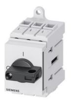
Load disconnector 3LD3, lu 16 A Main switch 3-pole Rated operating capacity at AC-23 A at 400V 7.5kW Installation in distribution boards, Basic switch with selector knob black
