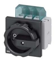
SENTRON, Switch disconnector 3LD, main switch, 3-pole, lu: 32 A, Operating power / at AC-23 A at 400 V: 11.5 kW, front-mounted, 1 NC, 1 NO, rotary operating mechanism, black, 4-hole mounting of the handle
