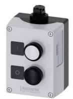
AS-Interface enclosure for command devices, 22 mm, round, Enclosure material plastic, enclosure top part gray, 2 control points plastic, Recess for labels, B=Pushbutton white, label: I, 1 NO, spring-type terminal, A=Pushbutton black label: O 1 NC, spring-type terminal, floor mounting, Insulation displacement system on top, Labels enclosed
