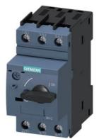
Circuit breaker size S0 for motor protection, CLASS 10 A-release 1.4...2 A N-release 26 A screw terminal Standard switching capacity
