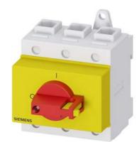
SENTRON, Switch disconnector 3LD, emergency switching-off switch, 3-pole, lu: 125 A, operating power / at AC-23 A 400 V: 45 kW, installation in distribution boards, knob-operated mechanism, Red / yellow, handle direct at the switch
