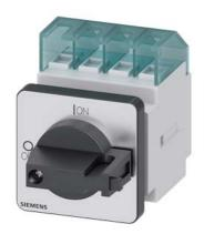
SENTRON, Switch disconnector 3LD, main switch, 4-pole, lu: 16 A, Operating power / at AC-23 A at 400 V: 7.5 kW, front-mounted, knoboperated mechanism, black, 4-hole mounting of the handle
