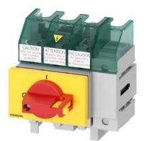
SENTRON, Molded case switch 3LD5 UL, Emergency switching-off, 4-pole, certified according to UL489 UL60947-4-1 and IEC60947-3, UL: 30A, SCCR 50kA at 480VAC, Operating power at 480VAC 3-phase: 20hp, IEC: 32A, Operating power at AC-23A at 400V: 15kW, floor mounting with direct handle, red/yellow, incl. terminal covers for the infeed side
