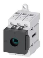
Load disconnector 3LD3, lu 40 A Main switch 3-pole Rated operating capacity at AC-23 A at 400 V 18.5 kW Installation in distribution boards, Basic switch without Knob-operated mechanism
